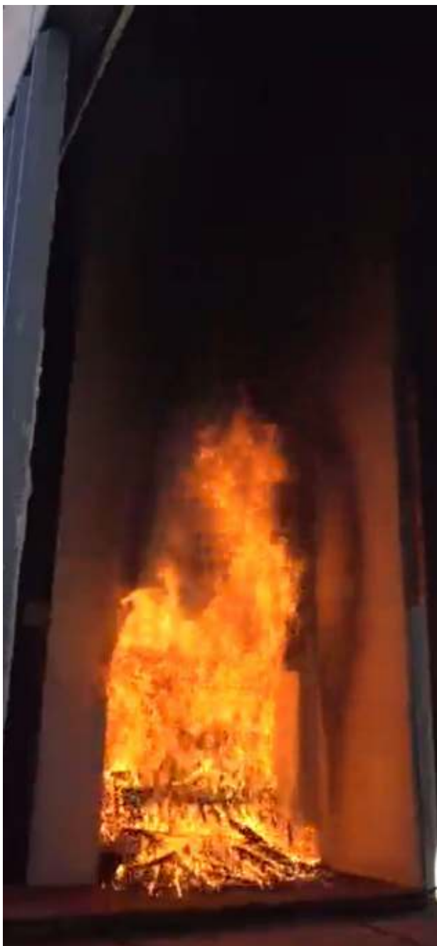
FIGURE 17: CRIB COLLAPSE AND 30 MINUTES
