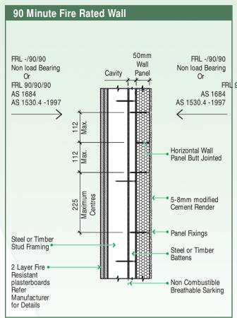
The Fire Rating information for sections 6.2, 6.3 and 6.4 are based on CSIRO Opinion FCO-2310 Dated 17th February 2004 and the Fire Resistance Test performed by Warrington Fire Research Consultancy Testing, WFRA Report No.2172500 of a 50mm thick QT ECOSERIES Exterior Wall Panel, system tested in accordance with AS 1530.4-2005 dated 01st May 2007.
