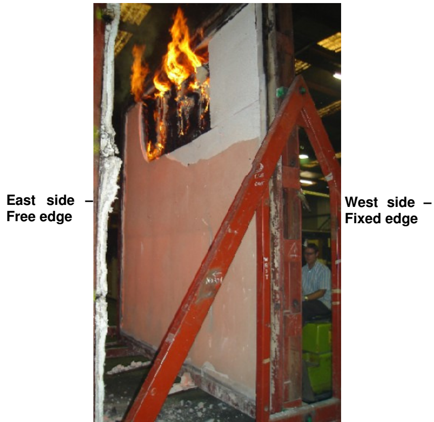
Figure A6.3 Exposed face of test specimen after the completion of the test.
